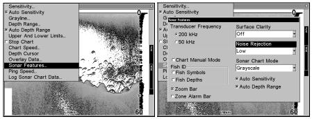
Sonar Menu with Sonar Features selected (left). The Sonar Features menu (right), Noise Rejection selected with ASP at default low setting. To change the ASP level:
